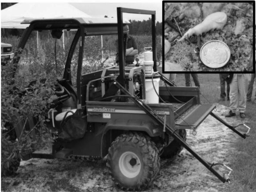
Figure 3. The mechanical applicator mounted on a 'gator' in a blueberry field. The applicator has two adjustable arms that protrude from the back of the gator towards the ground that contain valves that open and close periodically, at pre-set intervals and pre-set opening times, allowing the SPLAT® OrB under pressure in the pipes, to exit and fall onto the ground. By setting the SPLAT® OrB pressure, the time interval between openings, and the time that the valve is opened, the user is able to precisely deposit dollops at regular intervals simply by adjusting the speed of the vehicle. Inset shows a gray dollop of SPLAT® OrB near a US $0.10 coin, for scale.
